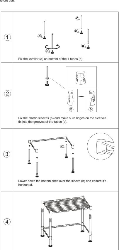
Fix the plastic sleeves (b) on top of tubes according to Step 2 and
