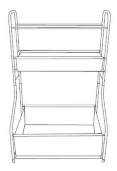
WARNING: DO NOT STAND OR SIT ON THIS CUBE UNIT. DO NOT CLIMB. DO NOT USE UNTIL ALL JOINTS ARE FIRMLY SECURED. USE ONLY ON A FLAT SURFACE. DO NOT DRAG WHEN MOVING THE PRODUCT TO AVOID DAMAGING THE JOINTS. MAXIMUM SAFE LOAD WEIGHT -TOP SHELF 3kg. MIDDLE COMPARTMENT 5kg. BOTTOM COMPARTMENT 10kg.
