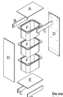
Do not tighten the screws fully during assembly. Fully tighten screws after the final assembly steps
