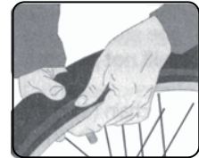
FIGURE F Use thumb to press valve stem through hole in rim. Make certain valve stem is straight.
