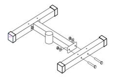
Step 2. Put right & left upright pole (3,4) on the part of step 1, then secure them with bolt, washer and nut (8,9,10). Insert the top cap (7) into the tube of right & left upright pole.
