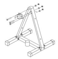
Step 4. Insert the 4pcs weight tube (5) into the hole of right & left upright pole, secure them with bolt (12). After this.
