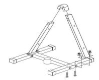
Step 3. Connect curl bar holder (6) and the part of step 2 together, then secure them with bolt, washer and nut (9,10,11)
