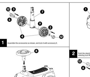
Push the steering wheel down onto the steering column ensuring holes on the steering wheel align with the clips on the steering column. Ensure this is a tight fit.
