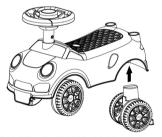
Push the stabilizer up through the hole in the main body. Ensure it locates securely in the underside of the body.
