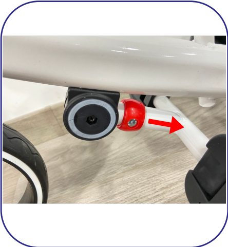
4. Pull the red ring down to fold and unfold the pedal
