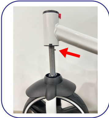
1. Install the front fender and insert the front fork to the main frame, silver button is backward
