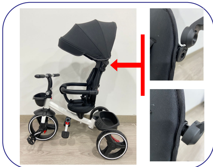
7. Install the canopy by inserting the buckle, adjust the angle of canopy by pulling out both buckles
