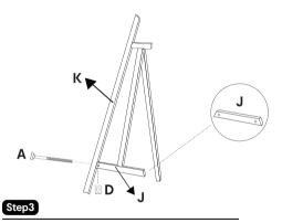
Fit part J into assembled unit as shown. Secure part K and J, using bolt A, washer and cam. Do not tighten bolt at this moment.
