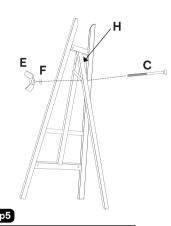
Secure support H, using bolt C, washer and wing nut, but do not over tighten the bolt. Assembly is now complete.
