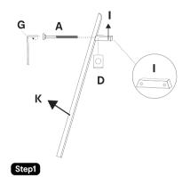
Assemble part K and I, using bolt A, washer and cam. Do not tighten the bolt at this moment.
