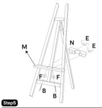
Attach the canvas support M and N to the assembled unit as shown. Secure using bolts B, washers and wing nuts, but do not over tighten the bolts.
