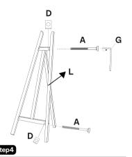
Fit part L into assembled unit as shown. Secure using bolts A, washers and cams. Now tighten all bolts using allen key.
