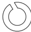
(27) Spring Washer \phi 19.5 \times \phi 11.5 \times 3 2PCS
