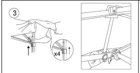
Engage the slider at each corner by pushing up with one hand while holding down the top of the leg with the other hand. A snap button will engage in the locating hole. Repeat this operation on the remaining three legs.
