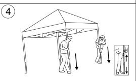
You and your partner should each place a foot on the foot plate of the bottom of adjacent legs and lift up the leg, sliding the inner leg out until the snap button will engage in the locating hole. Repeat this operation for the other two legs.
