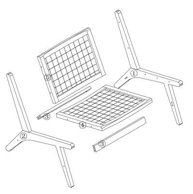
DO NOT TIGHTEN THE SCREWS FULLY DURING ASSEMBLY. FULLY TIGHTEN SCREWS AFTER THE FINAL ASSEMBLY STEPS.
