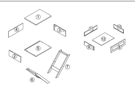
DO NOT TIGHTEN THE SCREWS UNTIL THE PRODUCT IS FULLY ASSEMBLED.
