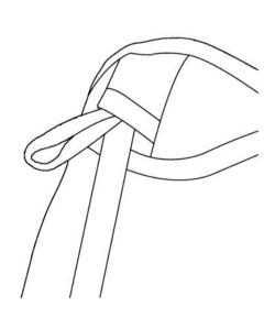
Step 3: Set up by pulling the corner loops and insert the tubes into fabric corner.
