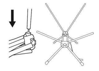
Step 2:Insert all tubes into the plastic parts.main frame is set up.
