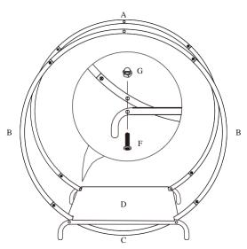
**Step 3.** Connect the top of the two circles using screw F and nut G (please see image below). You can decorate the stand once completed.
