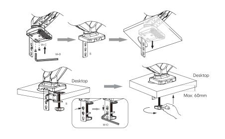
NOTE: If your desk has an existing grommet hole, please install directly. If there is no existing grommet hole, make a mark on your mounting surface, and use a drill to drill a hole (Dia 40-60mm) in the mounting surface.
