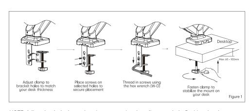
NOTE: Adjust the desk clamp clamping range using the adjustment hole. Position the clamp to the required thickness of the desktop (see Figure 1).
