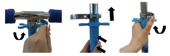
Step 3: Press the scooter handgrip on the steering bar until the bullets are in position. Adjust the steering bar by turning off the smaller ring with a key and centre handles at right angles to the front wheel. Clamp the ring again.
