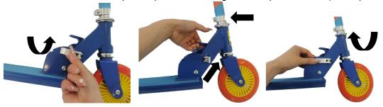
Step 3: Release the scooter handle by pressing the bullet.
