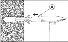
**Step 2:** Insert PART A into the hole
