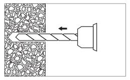
**Step 1:** PART A-screw size:M4,use a drill bit with the same diameter as PART A for drilling.
