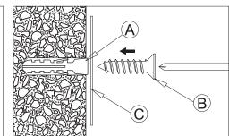
**Step 3:** Screw PART B and PART C into PART A
