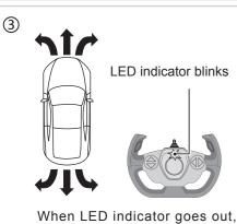
When LED indicator goes out, pairing process is completed.
