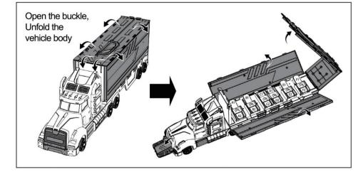
Step 2: Ejection racing mode (track installation diagram)
