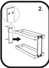
Put the second leg in place and screw together.
