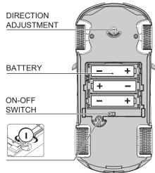
Function: Forward, Reverse, Turn Left, Turn Right. Features: Authentic car styling with injection moulded body, independent suspension system.
