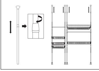
STEP 4 Stand the set of shelving up in the room and turn the plastic locker from the feet of the telescopic rods (G) clockwise direction to adjust the height of the poles to suit your environment. Please note that part (E) is for large height adjustments where as part (G) is for small height adjustment.
