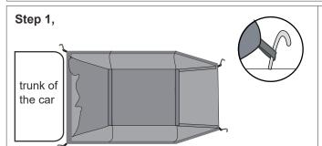
Lay the tent flat on the ground behind the vehicle, Secure the four corners with nails.
