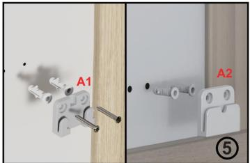
**Step 6.**Place B2 into A2 and B1 into A1. Make sure that A1 & B1, A2 & B2 is secured into their brackets properly.
