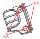
If you are securing all the brackets along the same surface, your screws need to be secured into holes A3A on the bracket.
