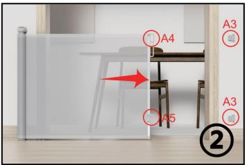
3. Make sure that A4 & A5 are hooked well into the A3 brackets.
