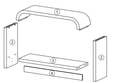
Do not tighten the screws fully during assembly. Fully tighten screws after the final assembly steps
