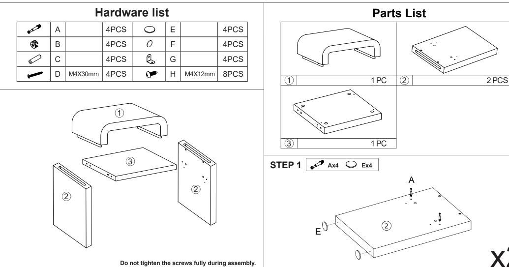
Fully tighten screws after the final assembly steps
