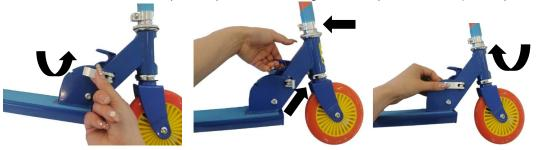
Step 3: Release the scooter handle by pressing the bullet.
