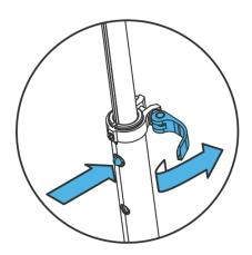
Step 2: Loosen the quick release (Open position). Pull the plastic lever up and lower the steering column backward until it clips into position, then tighten the quick release (Close position).
