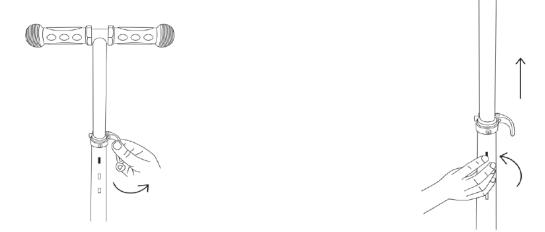
NOTICE: Always ensure handlebar is locked into place before use.
