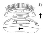
2. First, insert the right side of the brush pad into the buckle position, press the left side of the brush pad downward into the body you will hear a "click" if it is installed correctly.
