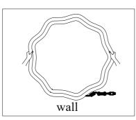
Align the hook on the back of the lamp with the nail and install it on the wall, then insert the DC plug into the socke on the lamp.
