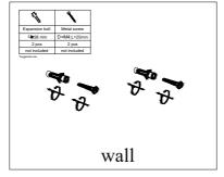
Insert the expansion bolts into the holes, make it smooth on the wall. Install the metal screws into the expansion bolts. Please make sure there is 3-5mm gap between metal screw and expansion bolt for hanging.
