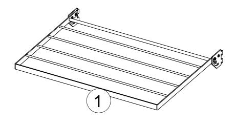
STEP 1 Install the laundry airer and apply a downward push to ensure it is locked in place.
