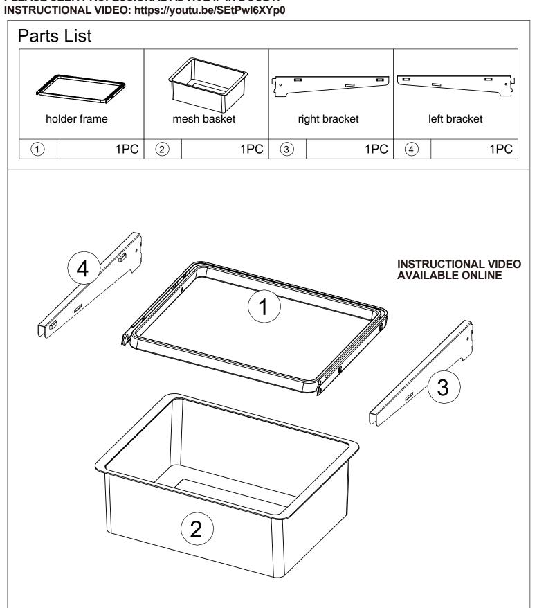
STEP 2 Install the holder frame and ensure that the snaps underneath the holder frame engage with the notches. Secure the holder frame and give it a push Install the left and right brackets and apply a downward push to ensure it is locked in place. STEP 1 to ensure it is locked in place.
