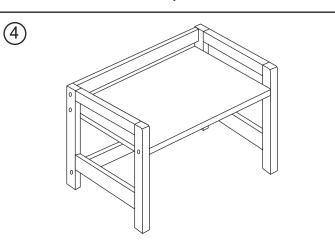
Note: If the bottom is uneven during installation, use a wrench to adjust the screw tightness to level it.
