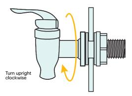
**Step 3** If the drink dispenser has any leaks, tighten the nut slightly to obtain a tighter seal.
