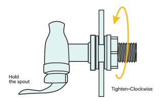
**Step 2** while holding the nut with one hand, turn the spout (through half a turn) clockwise with your other hand to tighten firmly.
