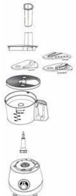
4. Place the lid onto the chopping jar and turn it clockwise until the tab of the lid clicks into slot in the jar handle. Make sure it is locked in position correctly, otherwise the appliance will not operate.
