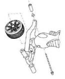
5. Turn dune buggy on it's side, place on a solid surface, capped side down. Place cap nut (B) in the cap nut tool and hold at the top of the axle (G). Using hammer, tap the cap nut tool until cap nut is securely fixed onto the axle.
