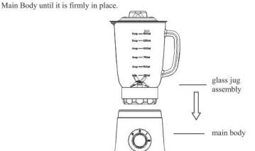
2. Place the Main Body on a flat, stable surface, and then place the assembled jug onto the top of the
