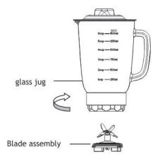
IMPORTANT! To prevent leaking DO NOT forget to place the sealing gasket.
