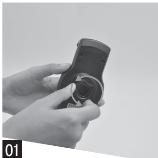
01 Step 1: Unscrew the nut behind the holder
