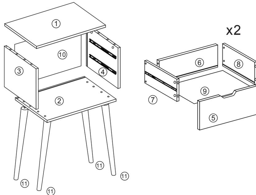
**Step 1:** Fix the screws from Part A onto board ①, and put Part B into the corresponding position (as per below diagram). Attach board ③ & ④ to board ①, and then fix the round screws from Part A with a screwdriver. Ensure all parts align.
