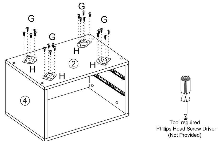
**Step 5:** Screw the legs (Part 11) into Part H from step 4.
