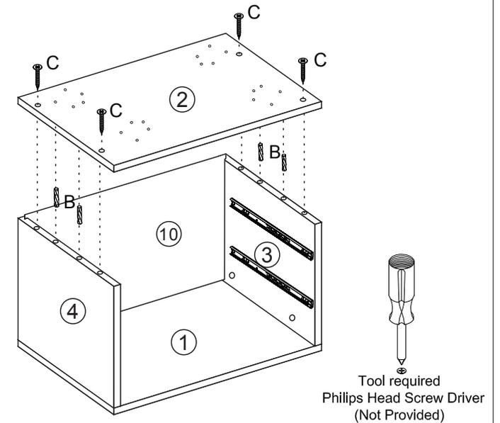
**Step 2:** Slide board ⑩ into the corresponding position (as per below diagram). Ensure it is fully fitted in the groove.
