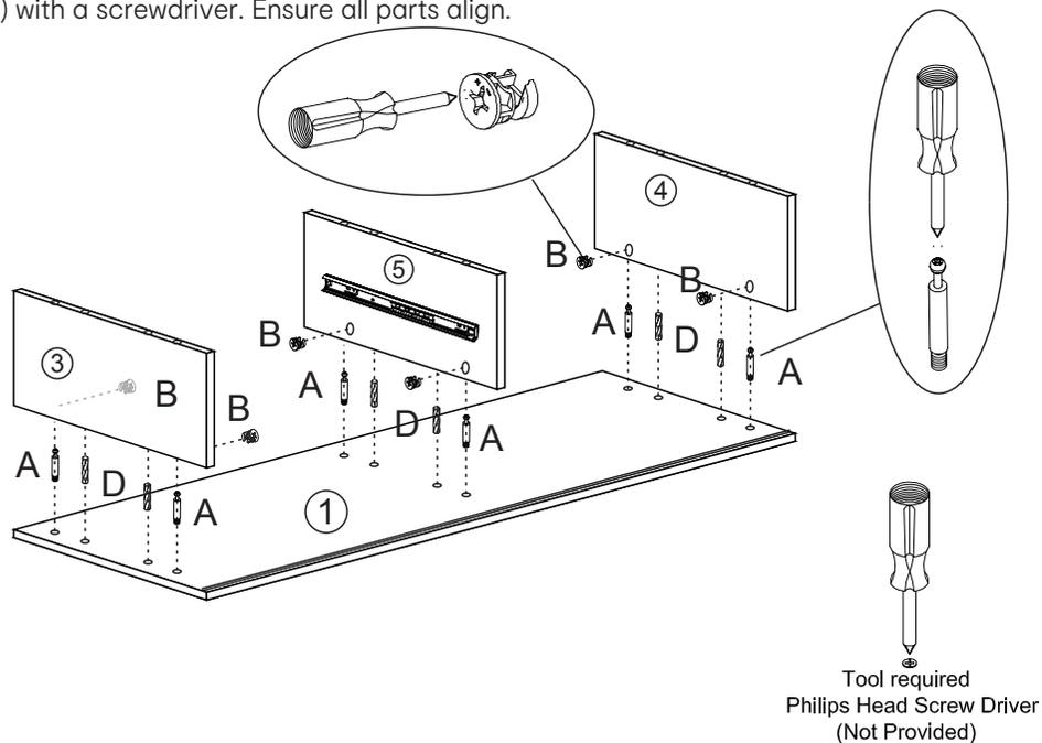
**Step 3:** Put part D into the corresponding position (as per below diagram) and attach board ② with screws (Part C). Ensure board ① is fully fitted in the groove.
