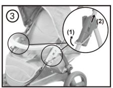
Move up the metal lockers and pull up the plastic lockers at the same time.
