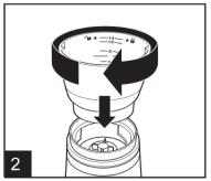
Twist grinding chamber clockwise to locked position. Make sure that the grinding chamber is FIRMLY locked into position.
