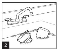
Wash cover and grinding chamber in hot, soapy water. Rinse and dry.
