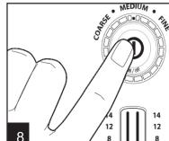
Move the cup selector to select the amount of cups to be brewed. Turn grind setting dial clockwise to select COARSE, MEDIUM, or FINE grind. Refer to charts on page 5 for grinding and cup selection. Press the ON/OFF (①) button to start grinding. It will switch off automatically after grinding.
