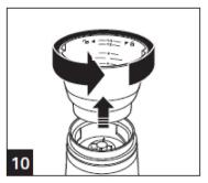
Twist grinding chamber counterclockwise to unlock; then lift straight up.
