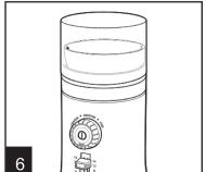
Place grinding cover onto grinder. Make sure the arrow on cover is aligned with the unlock symbol on back of grinder. Turn lid clockwise to locked position. Grinding cover will "click" when locked into position.
