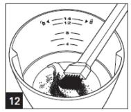
Use a small soft-bristle brush to remove grounds at the bottom of the grinding chamber.
