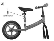
Push the seat post into the seat tube until it reaches the marker. Fix the screw tightly so the saddle doesn't move.
