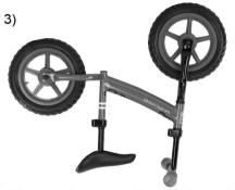
Turn bike upside down and rest the handlebars on the floor. Set the front wheel between the forks and fix the screw tightly. The safety pins of the washer must be placed in the designated hole.
