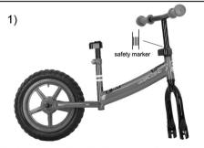
Push the stem into the front tube down to the marker. Fix the screw tightly so the handle bar stem is secured tightly and will not move.
