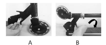
Step 3: Release the scooter handle by pressing the bullet.
