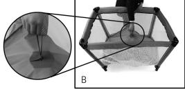
C Release each top rail by lifting the rail slightly and pressing the buttons located on the centre joint of rail.
