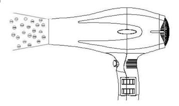
When you use the hair dryer, ion will be produced and released by the air flow. The Ionic Function generates a cloud of negative ions that can help to reduce frizz. Generally, flyaway, frizzy hair bears positive charge; the negative ions generated can neutralize the positive charge, eliminate static electricity and contribute to shine.
