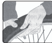
FIGURE F Use thumb to press valve stem through hole in rim. Make certain valve stem is straight.
