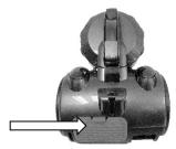
Unclip the grill by pushing down the clip and pull forward to expose the filter
