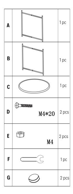
**Step 1:** Fasten leg tubes (Part A & B) by screws (Part D, E). Do not tighten all screws until assembly is complete.
