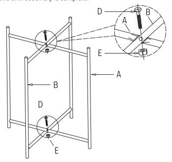
**Step 2:** Ensure all the screws have been tightened, put the table tray (Part C) on the leg frame (step 1), the assembly is completed.
